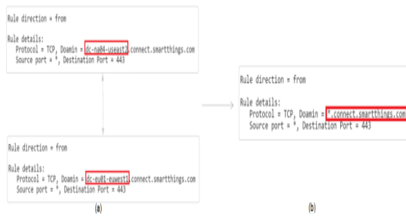
Figure 3: Two MUDs of SmartThings hub ACEs, one from the United States (top) and one from the United Kingdom (bottom). With the exception of the endpoint being.connect.smarthings.com, MUDIS's generic ACE (right) has the same parameters as the original.
